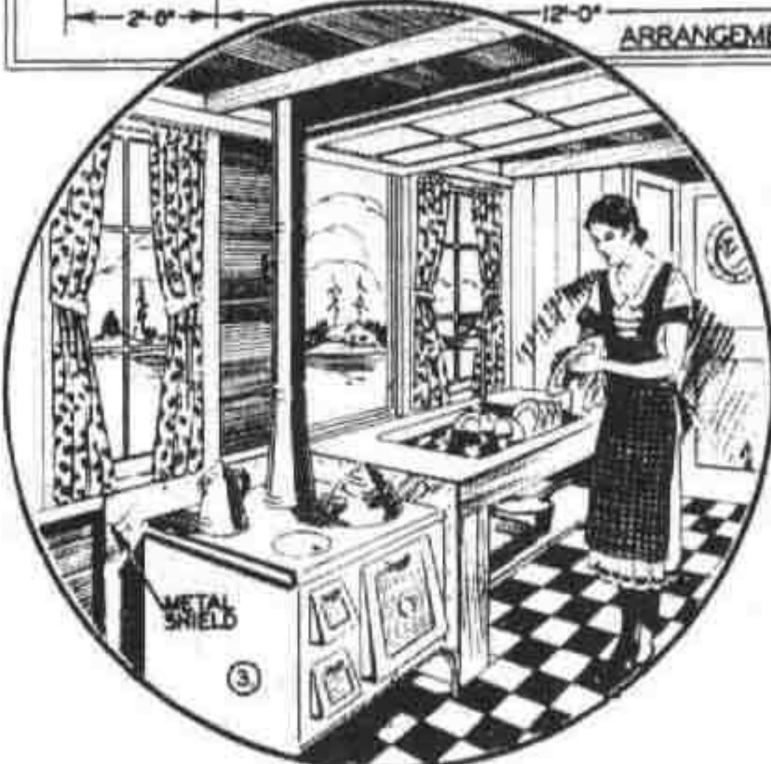
One corner of "Coolwater" house-boat showing kitchen range, sink, icebox. Windows are hinged to swing upward.
